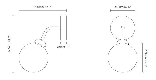
**Apiales Wall** is available with a classic wall plate or as a hard-wired version, to be connected directly to the electrical wiring in the wall. Wall plate fits US 3½" pancake bracket.
