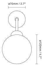
**Apiales Wall Hard-Wired** is connected directly to the electrical wiring in the wall. A classic wall plate version of the Apiales Wall lamp is also available.
