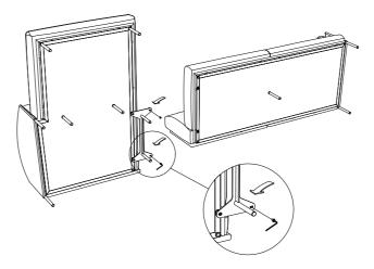
Joint bracket made of laser-cut steel sheet and steel rod, and steel rod feet Ø22 mm, screwed to the armrest structure with a bushings, welded within the structure and seat cushion support bar, in Ø20mm steel tube, fixed to the base by screw-spacer, with gunmetal grey epoxy powder coating.
